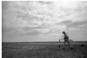
An Inforce team member strides back and forth across the desert, testing for underground soil disturbances, which might indicate a mass grave, with a magnetometer
